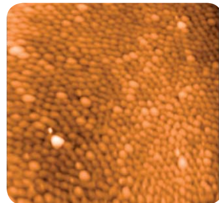
Figure 5 A scanning probe microscope allows you to see the aluminum particles in the foil.
